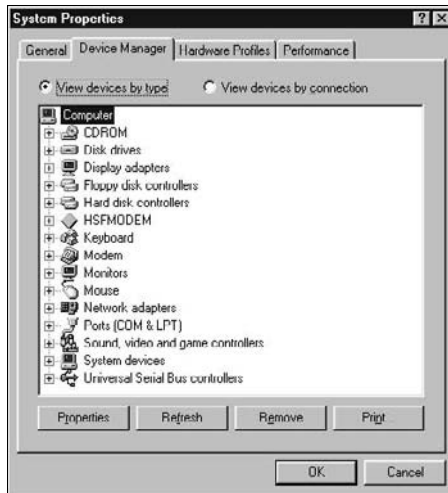
Figure 2-9: In Windows 98, the Device Manager gives you information on the hard- ware you've installed.
